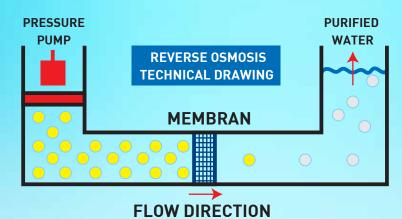
Reverse osmosis system allows converting highly contaminated surface water and sea-water into safe, potable and drinkable quality water. Reverse osmosis technology is being utilized by drinking water bottlers and household users. BİMAKS, designs and produces special chemicals which will increase the operational efficiency of all types of reverse osmosis systems. Through our products; we reduce our customers' costs and increase the life cycles of expensive filter membranes.
